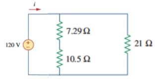
Now combining the 7.29  $\Omega$  and 10.5  $\Omega$  in series and then with the 21  $\Omega$  in parallel yields an equivalent resistance of 9.63  $\Omega$ , so  $i = \frac{120 \text{ V}}{9.63 \Omega} = 12.5 \text{ A}.$
