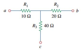
Using the Wye-Delta equations with  $R_1 = 10 \Omega$ ,  $R_2 = 20 \Omega$ , and  $R_3 = 40 \Omega$  yields
