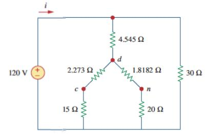
At this point series and parallel combining yields the same result as above. In a similar way one could start by converting the Delta formed by nodes c, n, and b to a Wye and then use series and parallel combining.
