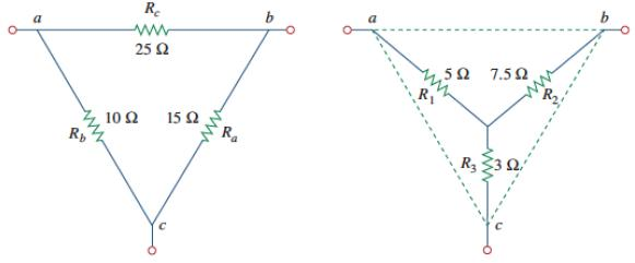
Using the Delta-Wye equations with  $R_a = 15 \Omega$ ,  $R_b = 10 \Omega$ , and  $R_c = 25 \Omega$  yields
