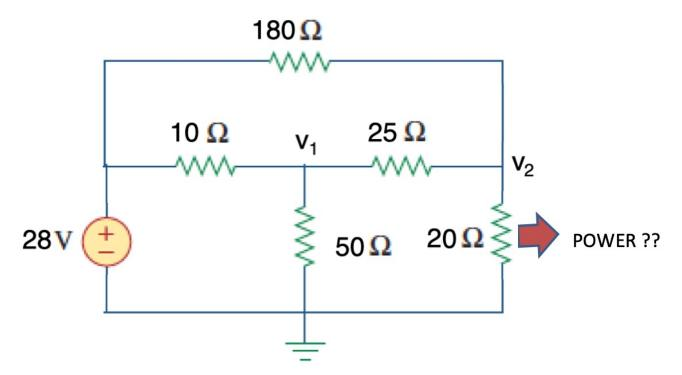
• How much power is dissipated in the 20  $\Omega$  resistor? — Method: node analysis  $\rightarrow v_0 = 10$  V
