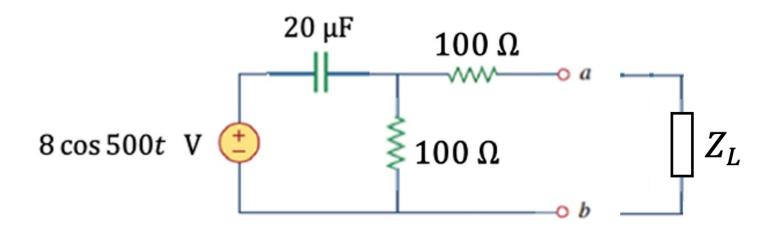
Since  $V_{Th} = 4\sqrt{2} \cos(500t + 45^\circ) V$  and  $Z_{Th} = 150 - j50 \Omega$ , then  $Z_{Th} = 150 + j50 \Omega = 150 \Omega$ , 0.1 *H*, and P = 26.7 mW
