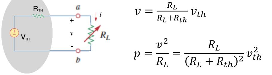
•  $\frac{\partial p}{\partial R_L} = 0$  yields a max of  $P_{max} = \frac{V_{th}^2}{4R_{th}}$  when  $R_L = R_{th}$
