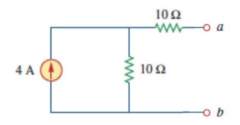
**Example:** find the load that dissipates maximum power
