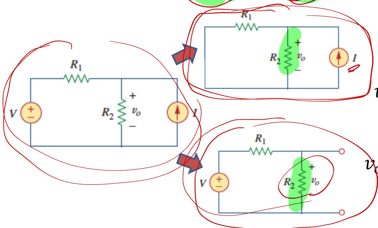
$$v_o(I, 0) = \frac{R_1 R_2}{R_1 + R_2} I$$
