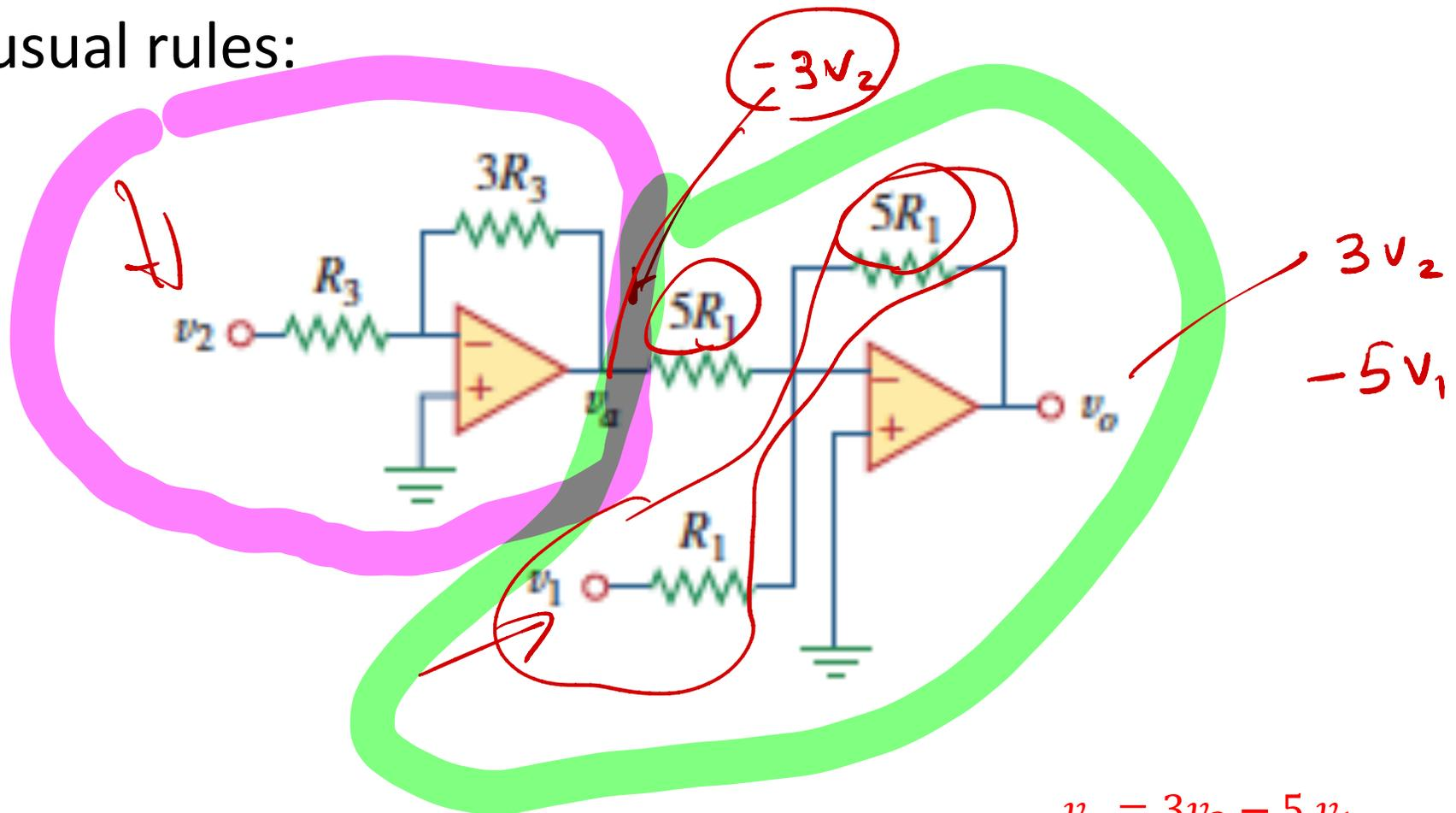
$$v_o = 3v_2 - 5v_1$$
