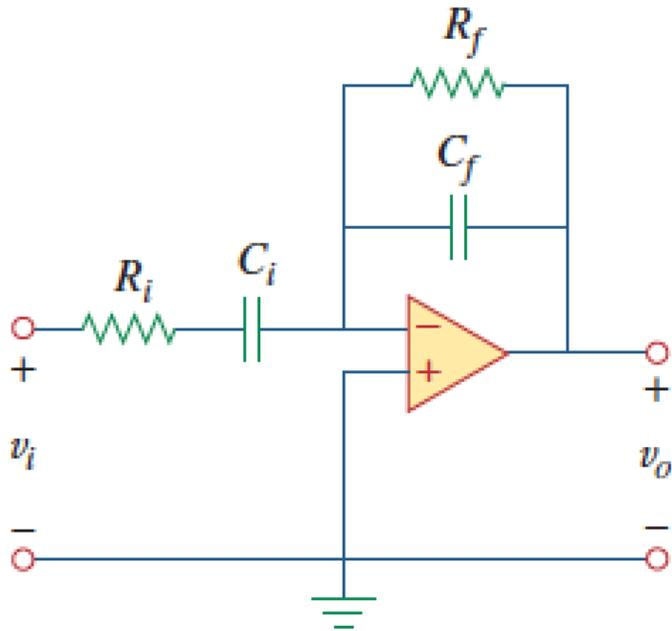
$$v_o(t) = \frac{A\omega R_f C_i}{\sqrt{1+\omega^2 R_i^2 C_i^2} \sqrt{1+\omega^2 R_f^2 C_f^2}} \cos(\omega t + 270^\circ - \tan^{-1}(\omega R_i C_i) - \tan^{-1}(\omega R_f C_f)) \text{ V}$$
