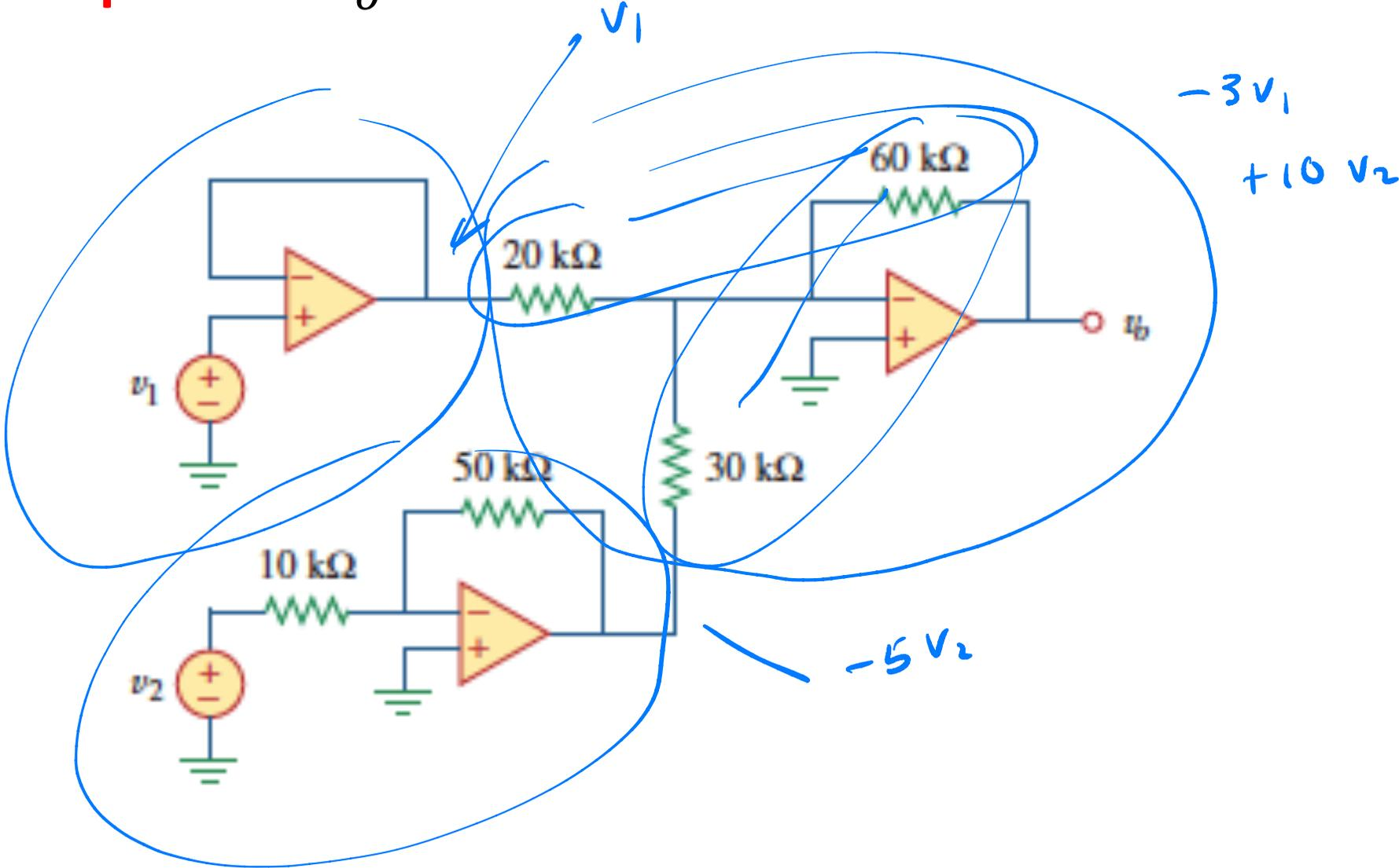
$$v_o = 10v_2 - 3v_1$$
