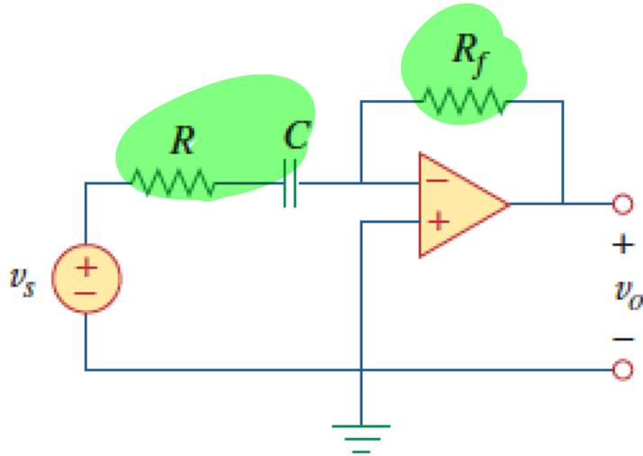
$$V_o = - \frac{V_i C}{R_f} \frac{R_f}{j\omega C}$$
