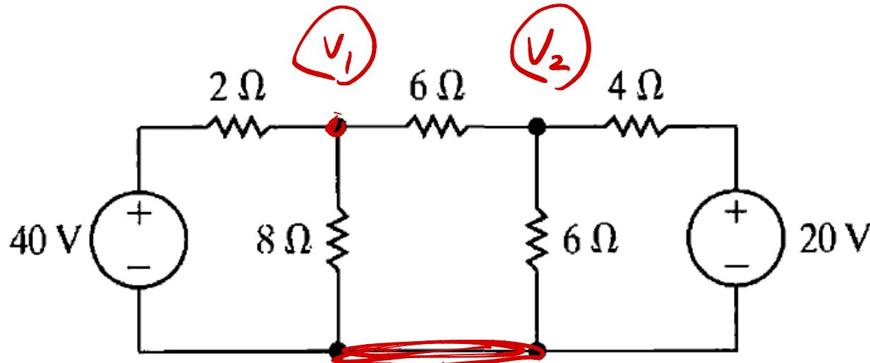
node  $v_1$ :  $\frac{v_1}{8} + \frac{v_1 - v_2}{6} + \frac{v_1 - 40}{2} = 0$
