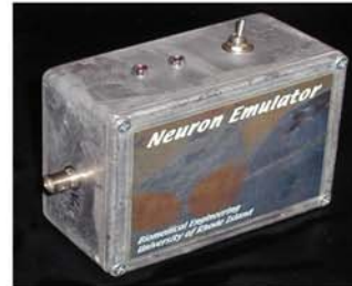
Figure 4. The neuron emulator performs real-time, interactive simulation of a neuron in terms of the following: 1) electrode and membrane resistance and capacitance for both current input and voltage output ports (figure 4), 2) membrane resting potential when input current is zero, 3) firing of action potentials above a depolarization current threshold, 4) adaptation of the spiking response (figure 5), 5) hyper-polarization following each spike, and 6) response to voltage clamping.
