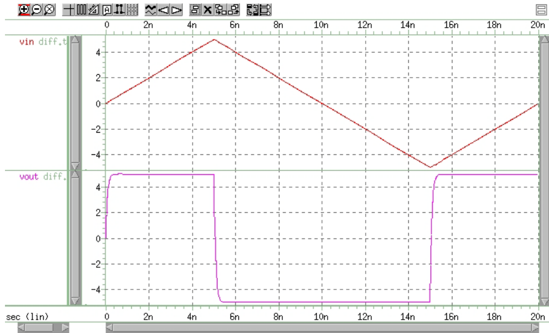
Figure 209 Response of a Differentiator to a Triangle Waveform
