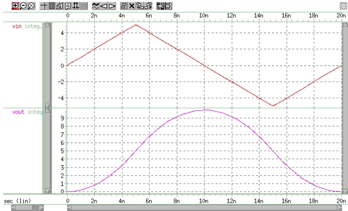
Figure 207 Response of Integrator to a Triangle Waveform
