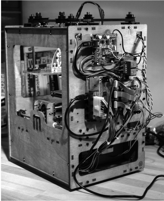
Figure 1-5. MakerBot CupCake 3D printer with Arduino-compatible electronics
